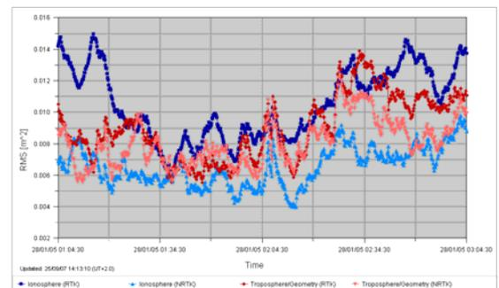
**Figure 2 - Leica SpiderQC, Example of Global RMS for Ionosphere & Troposphere, for RTK and NRTK**
