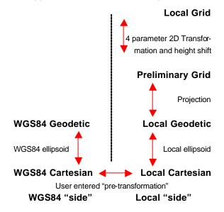
Note, when using a TwoStep transformation it is not possible to see the "preliminary grid" coordinates either in LGO or on the System1200 instruments. Only the final local grid coordinates are shown. This is correct since the "preliminary grid" coordinates have no practical use.
