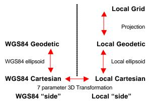
The advantage of the Classical 3D transformation is that it is the most rigorous transformation type - it is a similarity transformation, which keeps the full geometrical information. The disadvantage is that that knowledge of the local ellipsoid and the map projection is
